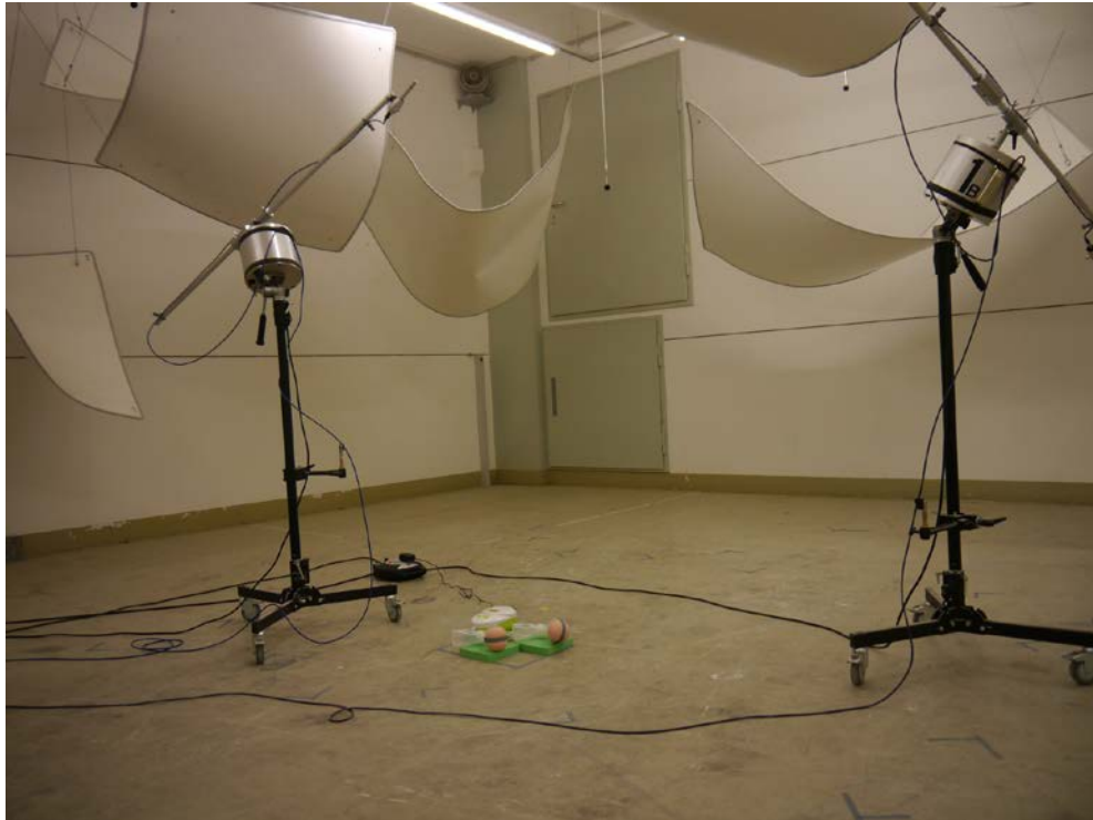
Figure B.3. Test arrangement on the reverberation room floor.
